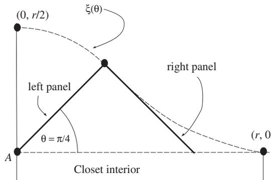
**Figure 2** This figure shows the view from above a bifold door as the door closes. It first sweeps out the area under the circular arc of radius  $r/2$ , but when  $\theta$  reaches  $\pi/4$  the nature of the curve changes. Notice that “bifold” is a misnomer. There is only one fold.
